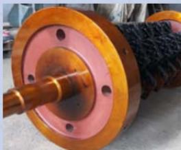
**LEVELLER ROTOR ASSEMBLY**
