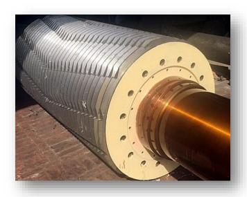
Chevron shaped grooves are cut lengthwise through the circumferential grooving as an aid to feeding. Such grooving decreases the effective pressure surface of the rollers and causes excessive bagasse in mixed juice. We offer rollers with arcing & Chevron grooving as per need of customer.
